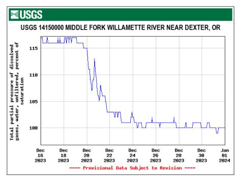
Figure 50. Total Dissolved Gas Saturation (%); Middle Fork Willamette River, Near Dexter, OR.
