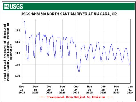
Figure 20. Total Dissolved Gas Saturation (%); below Big Cliff Dam.
