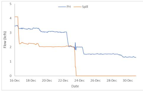
Figure 22. Hourly Flows PWR vs. Spill (Big Cliff Dam).
