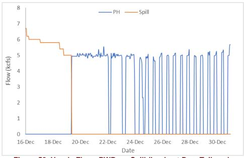
Figure 58. Hourly Flows PWR vs. Spill (Lookout Dam Tailrace).
