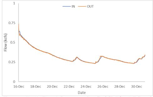
Figure 46. Hourly Flows Inflow vs. Outflow (RO) (Fall Creek Tailrace)
